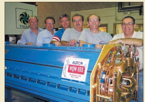
The ALSTOM Canada assembly team beside the last of the 52 twin-aperture "warm" quadrupole magnets delivered to CERN in 2003. (Courtesy Yvon Langevin, ALSTOM Canada.)
