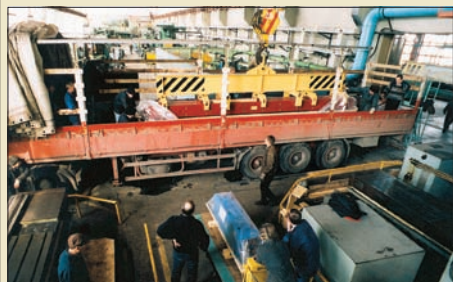
Loading a 6 m dipole magnet prior to the 6000 km journey from Novosibirsk to CERN in 1999.
