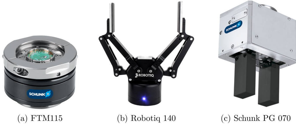
Figure 3.6: The force-torque sensor and two different end-effectors of the Schunk Powerball robotic arm
