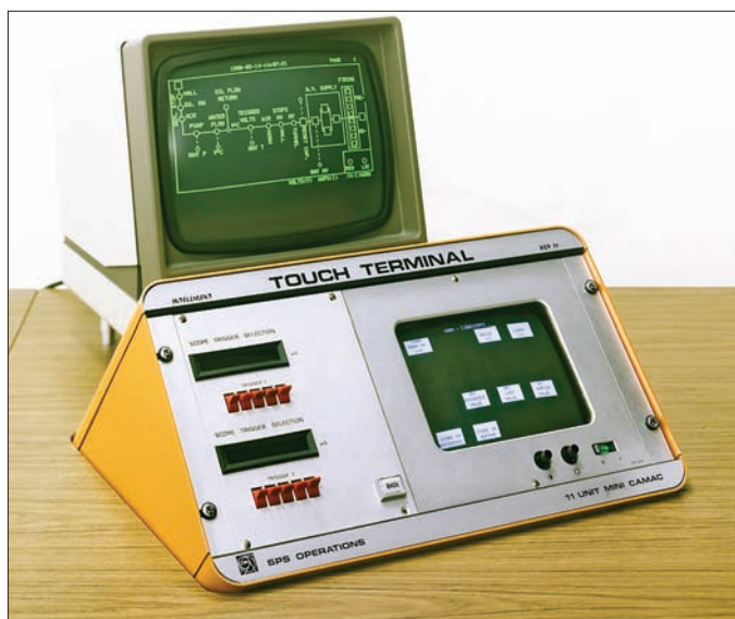
The Touch Terminal as developed for the Antiproton Accumulator (AA).
