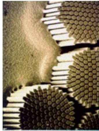
(b) Filament in Rutherford cable [13]
