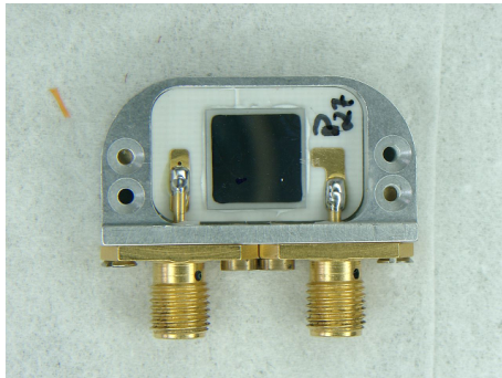
Figure 3.2: The BCM2 diamond ( 1\text{cm}^2 ) in its housing. The wire bonds to the metalization can be seen on the right hand side of the diamond.
