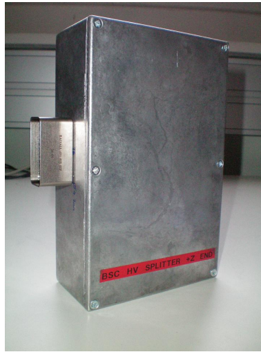
Figure 5.8: Photo of the high voltage splitter box with the 23 pin Radial connector. The box will be mounted under the HF platform.
