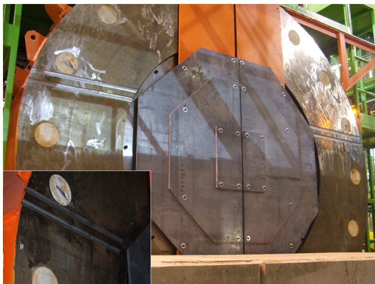
Figure 5.6: Photograph showing the two pairs of grooves cut into the HF outer steel rims to allow the exit of the BSC1 optical fibres. The grooves were positioned in a way to reduce Cherenkov radiation in the optical fibres and do not allow a direct line of sight to the beam pipe from the outside.
