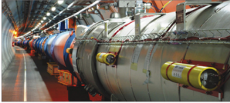
FIGURE 3.1: Beam Loss Monitor installed along the LHC ring
