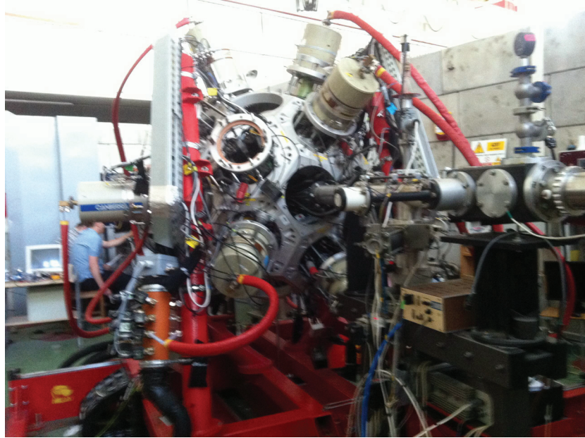
Figure 4.2: The EAGLE array with 12 HPGe detectors.
