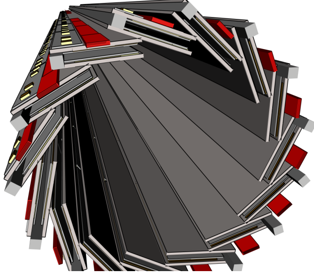
Figure 3.17: IGUANA representation of the stacked pixel layer geometry in a tilted configuration.
