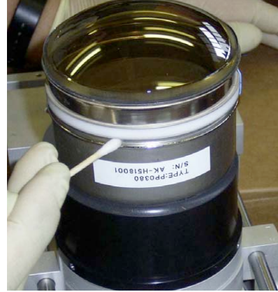
Figure 4.2: Photograph of an HPD, undergoing cleaning as part of the routine inspection procedure.
