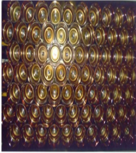
Figure 4.6: Photograph of close-packed hexagonal arrangement of HPDs in the RICH1 detector.
