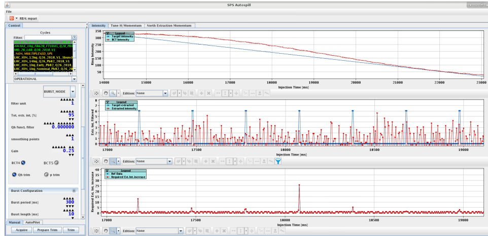
Figure 3.23: Example of the high level of noise on the measured spill (red curve, middle plot) during the burst mode slow extraction Autospill test.
