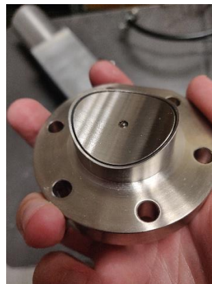
Figure 1: (Left) Test bench device used for measurements including two button BPMs on the opposite sides, “beam” propagation from left to right. (Right) A button BPM.
