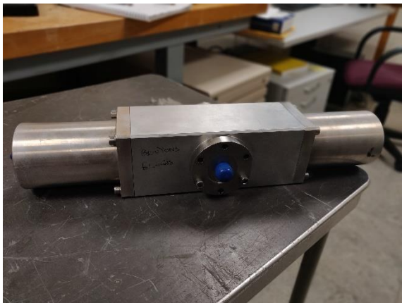
Figure 1: (Left) Test bench device used for measurements including two button BPMs on the opposite sides, “beam” propagation from left to right. (Right) A button BPM.
