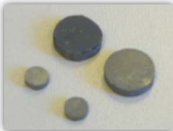
Figure 20 Samples prepared for the thermal conductivity measurement by the LFA 427 in both directions; longitudinal and transversal
