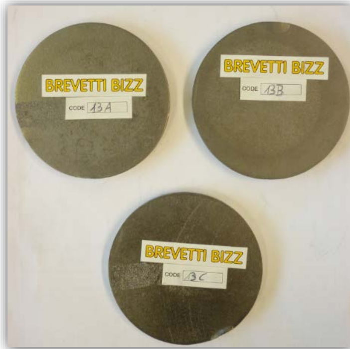
Figure 34 Compressed Al / Gr plate after Rapid Hot Pressing
