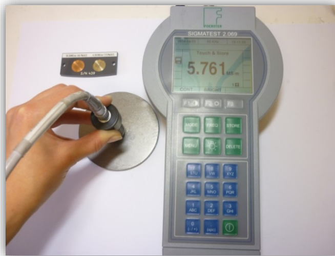
Figure 23 SIGMATEST 2.069 for electrical conductivity measurements
