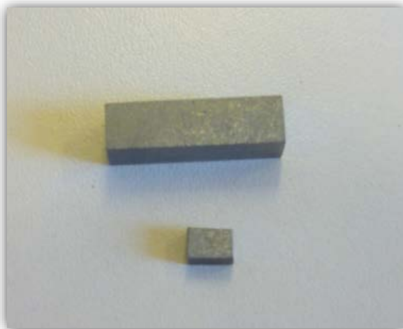
Figure 16 Al/C samples prepared for the CTE measurements
