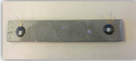
Figure 22 Sample prepared for the thermal conductivity measurement (on the in-house built device)
