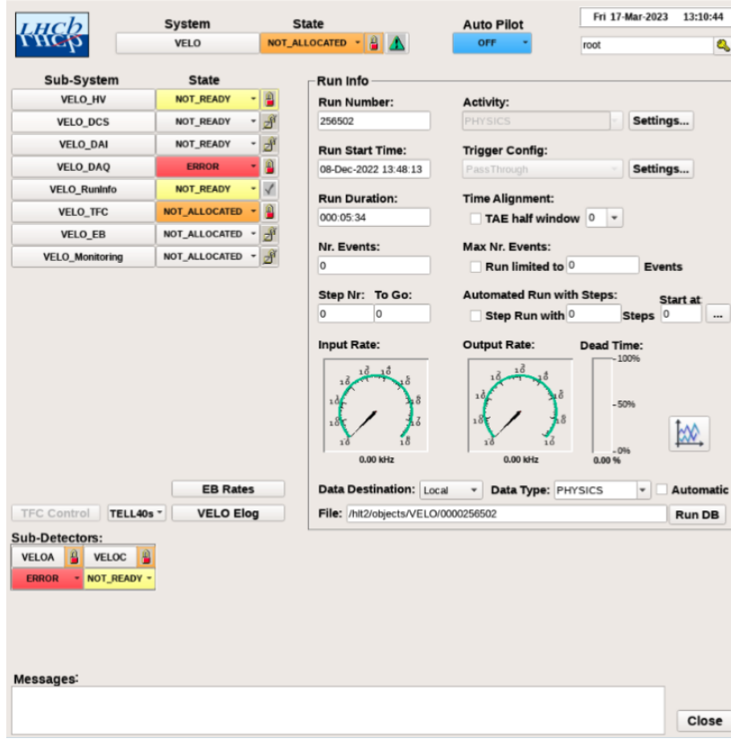
Figure 3.32: The upgraded VELO's Run Control panel. Each sub-system represents a control unit controlling a major part of the VELO detector, which can be accessed from this top panel. The state of the different control units can be seen as the coloured blocks. The panel also contains options to configure a local data-taking run.
