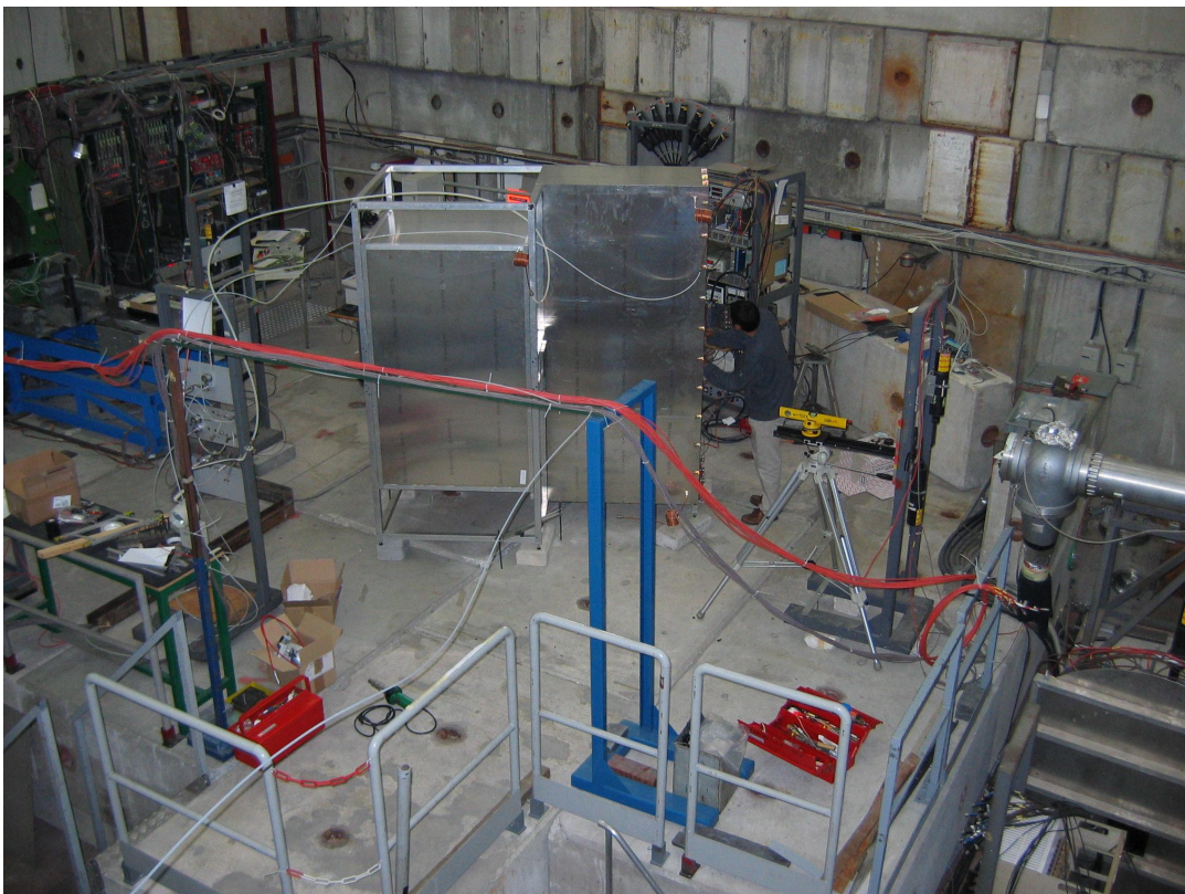
Figure 3.2: Photograph of the testbeam experimental area, showing the beam line and prototype RICH detector.
