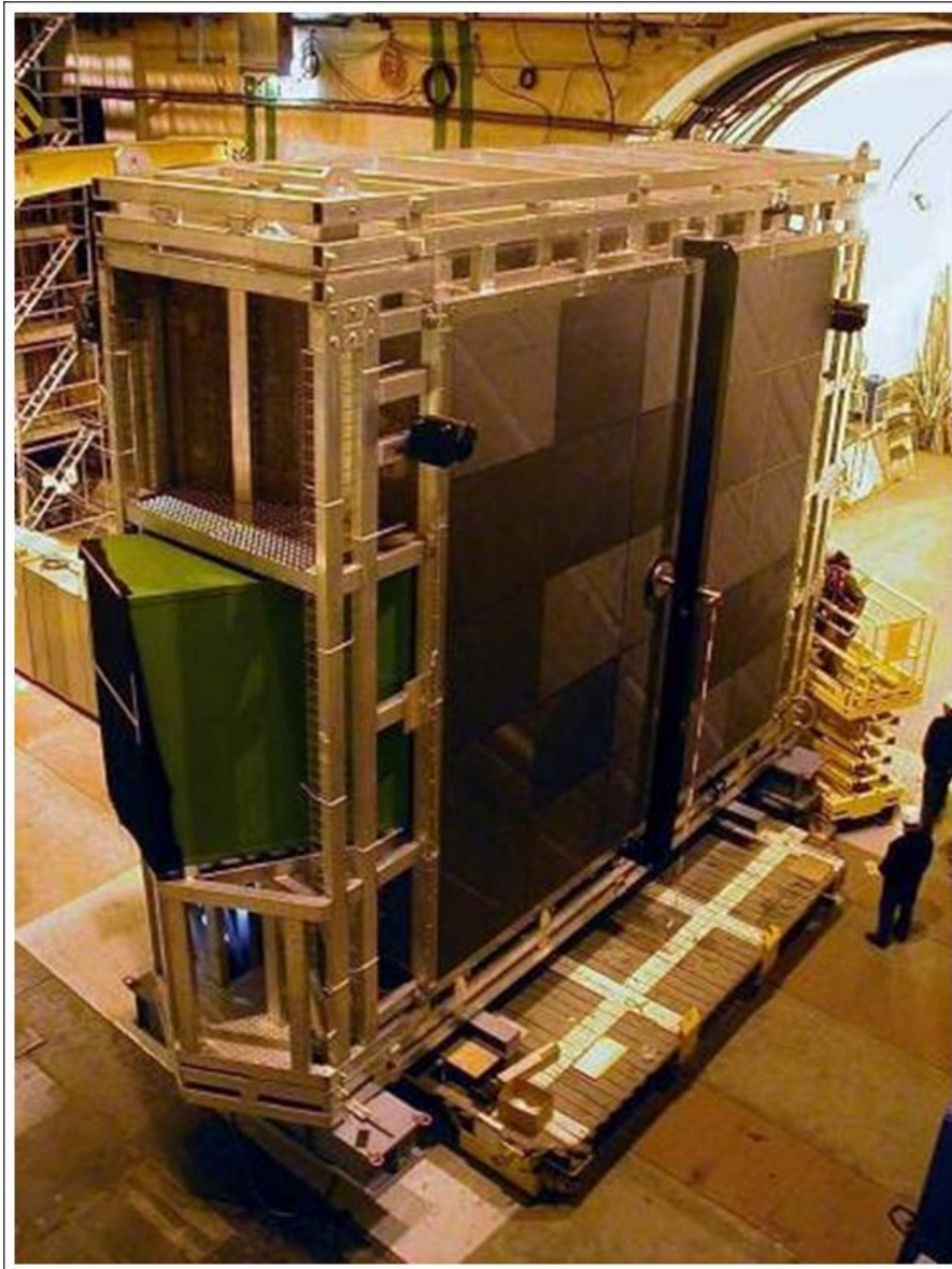
Figure 2.18: A photograph of the RICH2 detector under installation in the detector cavern.
