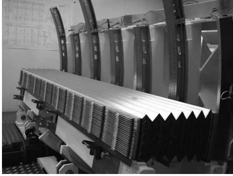
Figure 3.6: The partially constructed Liquid Argon calorimeter, showing the accordion structure [12].
