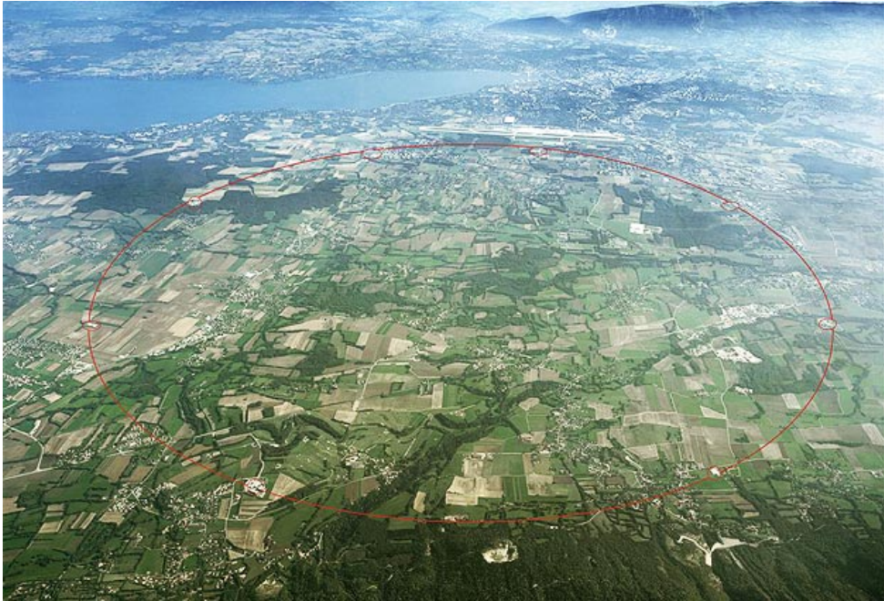
Figure 3.1: Areal view of the LHC ring in the region of Geneva. The red line marks where the tunnel is hosted underground, small circles indicate where the experiments are located. From [38].
