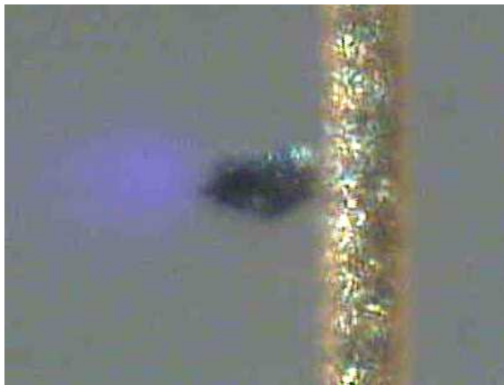
Figure 4.18: Tip induced discharge observed at the microscope
