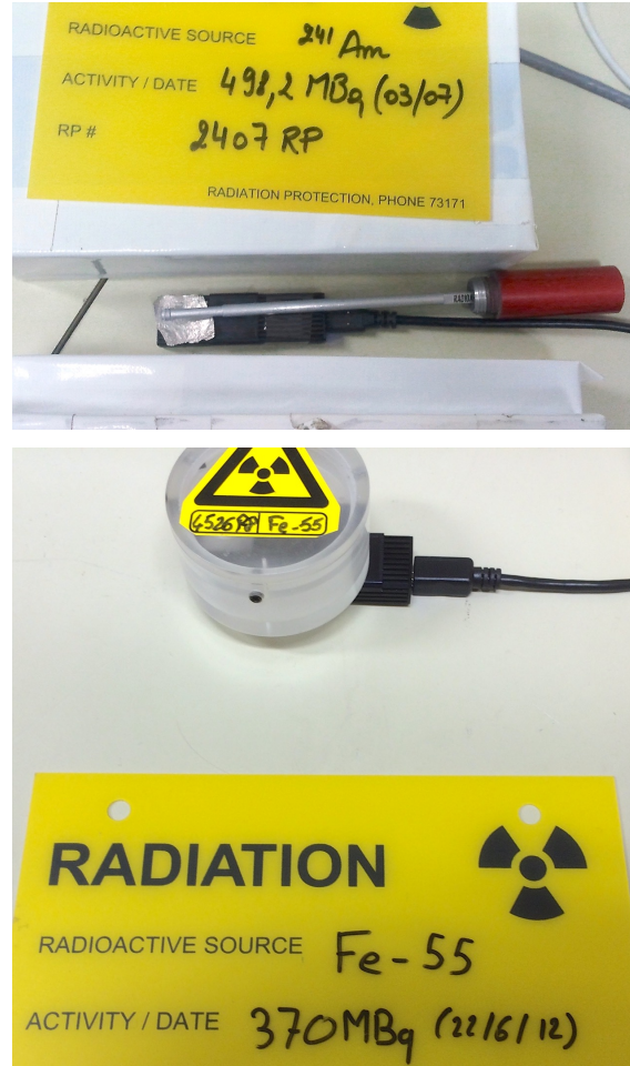
Figure 2.24: The upper measurement setup shows the ^{241}\text{Am} source (positioned at the end of the stick with the red handle) irradiating through a small window on the indium foil which is placed on the Timepix detector underneath. The white blocks are lead shielding covered with tape. The lower picture shows the ^{55}\text{Fe} source sealed in acrylic glass.
