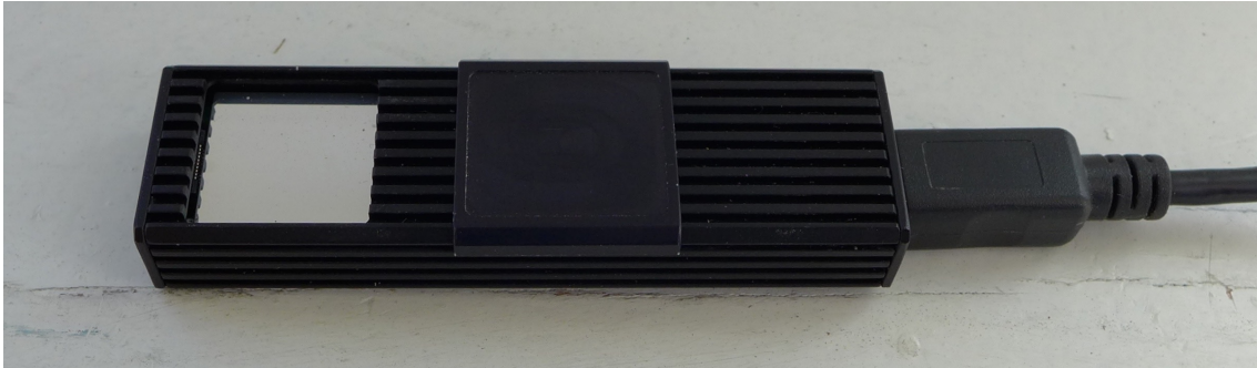
Figure 2.16: The USB Lite Timepix readout, measuring 1 \times 2 \times 6.8 \text{ cm}^3 with a mini-USB cable attached. The slider in the middle can be moved towards the left to protect the sensor.
