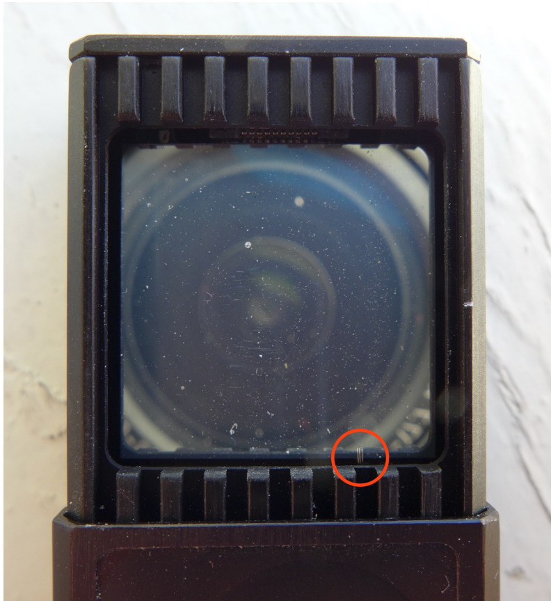
Figure 2.18: USB Lite readout equipped with Timepix and a 1.4 cm \times 1.4 cm sensor on top. The circle on the lower right marks the three bond wires that supply the bias voltage. 5
