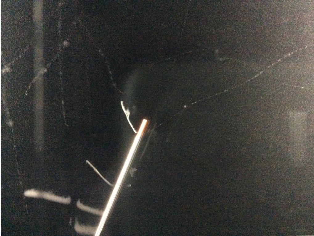
Figure 1.1: A weak radioactive welding stick in a cloud chamber emitting ionising radiation (tracks on the left side of the stick). The stick is made of tungsten and enriched with 4 % of thorium, which is an \alpha , \beta and \gamma -radiation emitter.
