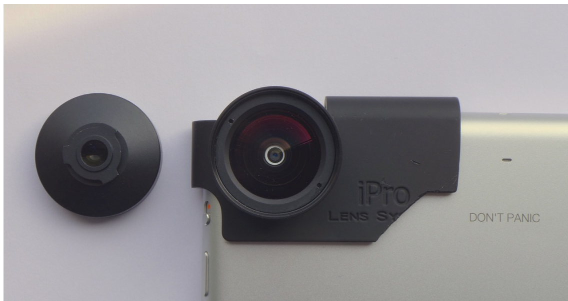
Figure 3.3: The iPro wide angle lens attached to an iPad mini with a modified clip. On the left side is the super wide angle lens showing its bayonet fitting.
