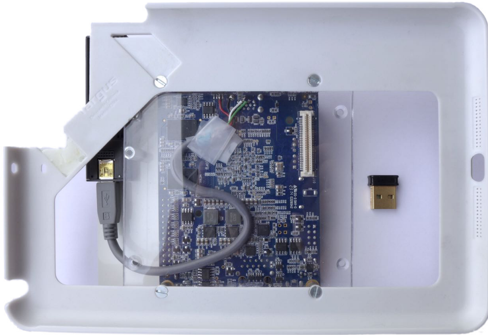
Figure 3.8: View on the back side of the modified cover, which is hosting an iPad mini during operation. The USB Lite is attached to the MinnowBoard Max via a soldered mini-USB cable. The small USB device on the right is the selected WiFi dongle.
