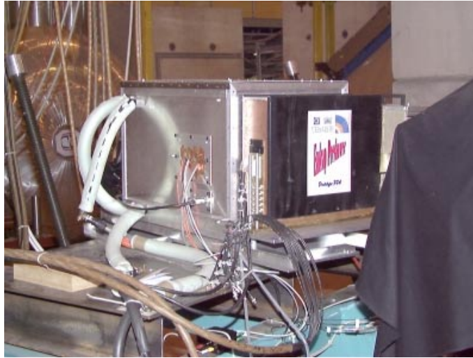
Figure 3.22: Photograph showing the Preshower prototype placed in front of the ECAL endcap box.
