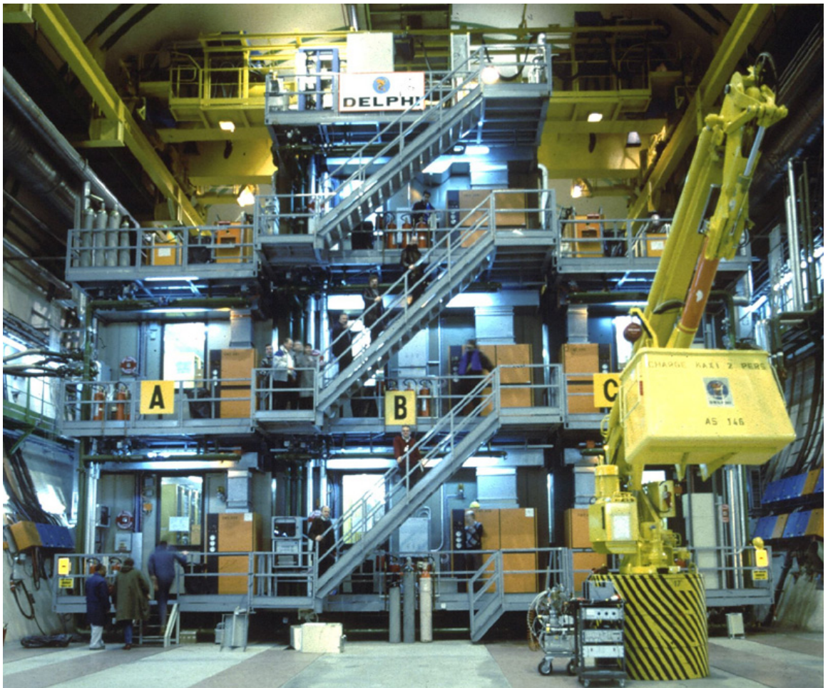
Figure 2.3: The DELPHI experimental hall. This view shows the counting houses, which are in front of the detector itself.
