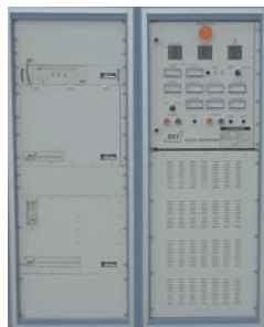
25KW, 18-32MHz, CW, Water Cooled, RF Amplifier
