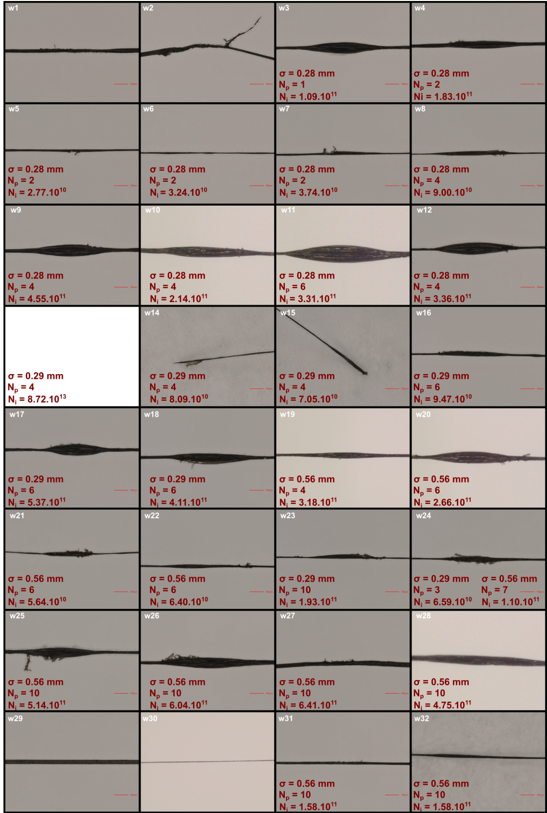
Figure A.4: Wires after irradiation with rea measured beam size ( \sigma ), number of pulses ( N_p ) and number of interactions ( N_i ).
