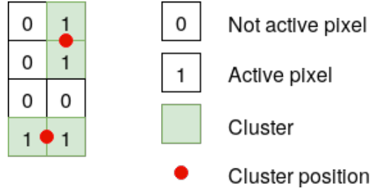
Figure 4.3: Example of isolated SP containing two clusters.
