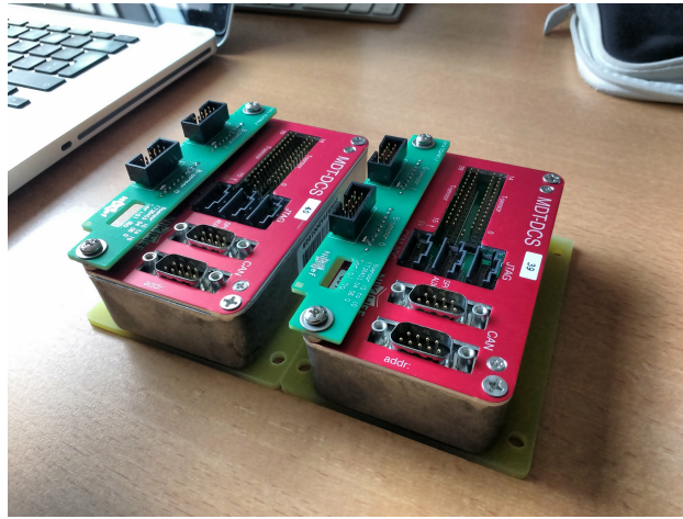
Figure 4.8: Two MDM boxes with ELMB, side by side. Each has two slots for B-field sensors, 30 slots for temperature sensors, and a few more slots for JTAG and SPI communication. Connection is based on CANbus, and allows daisy-chained schemes [20].
