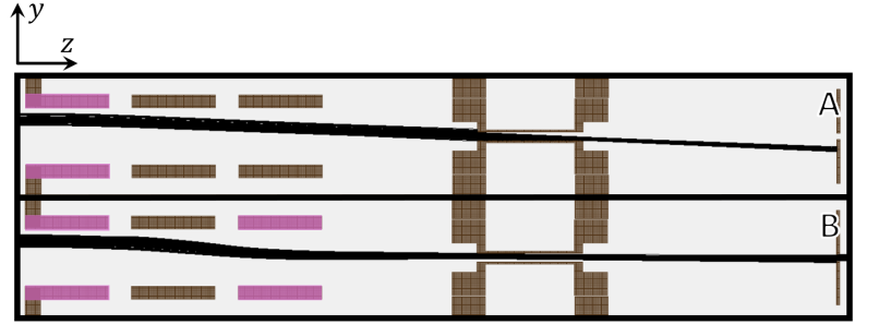
Figure 21: 0.5^\circ misalignment acceptance of 5 keV beam at focusing region - single (A) vs. double (B) steerer cases. Steering electrodes marked in pink.
