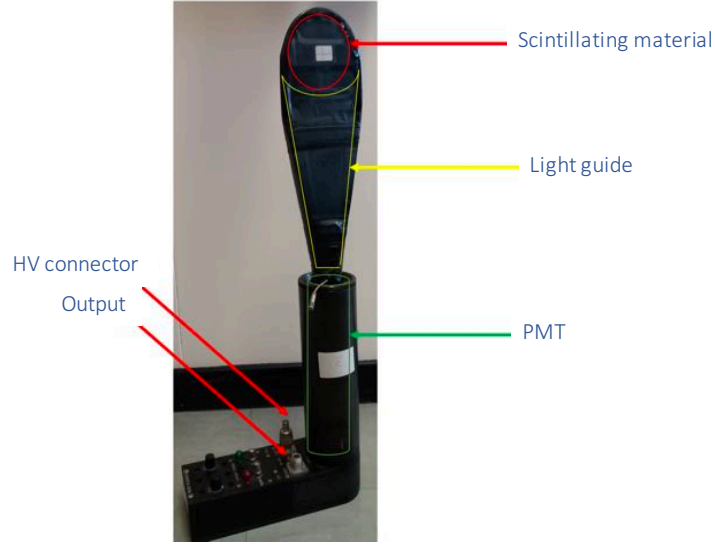
(a) Beam loss monitor before installation; main components are highlighted.
