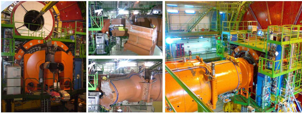
Figure 5.36: First closure of the forward region of CMS where T2 is installed. Left: The platform on two risers, ready to be moved on final position. The Hadron Forward, T2 and Castor are in open position to allow the insertion of the beam pipe. Middle: First Closure of the rotating shielding. Right: Forward region completely closed.
