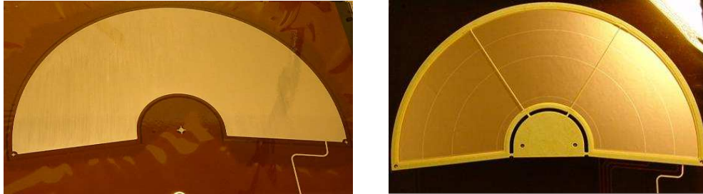
Figure 2.13: Left: The drift foil. It is realized with a polyimide foil with a 5\mu\text{m} copper cladding on a single side with thickness of 50\mu\text{m} glued to the front plate. Right: The GEM foil. It is realized with a 5\mu\text{m} copper cladding on both side with thickness of 50\mu\text{m} . The shape of the holes is double conical like in fig. 2.8. The diameters of the holes in the middle of the foil and on the surface are 65 and 80\mu\text{m} respectively. The distance between them is 140\mu\text{m} . The foil is characterized by a single plane in one side and by four electrically separated ring segments (visible in the picture) in the other. This reduce the risk of damage in case of discharge because not all the energy stored in the GEM foil will be released, but only the part of the sector involved. The foils are stretched and glued over supporting frames, which are manufactured by Computer Numerical Control (CNC) machining from fiberglass reinforced epoxy plates (Permaglas) with thicknesses of 2\text{mm} . Two additional supporting spacers of thickness 0.5\text{mm} are designed in the middle of the frames. Their position is slightly asymmetric to minimize dead areas. In the picture it is shown one foil with its spacer.
