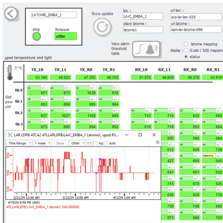
Figure 3.38: DCS panel for monitoring the light power of data fibers.
