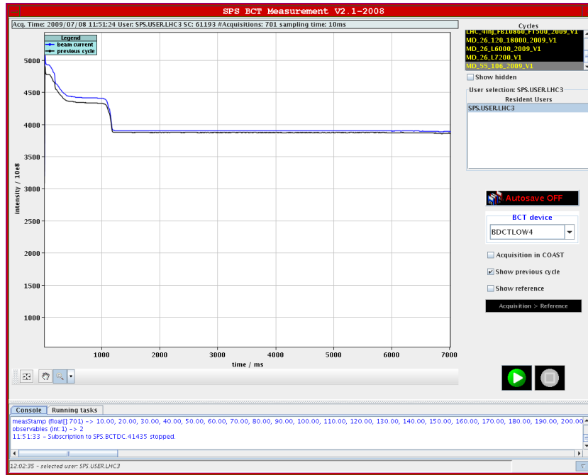
Figure 4.27: The beam structure used in the SPS experiment observed from the monitor of Fast Beam Current Transformer: four bunches with 5 - 6 \cdot 10^{10} protons per bunch.
