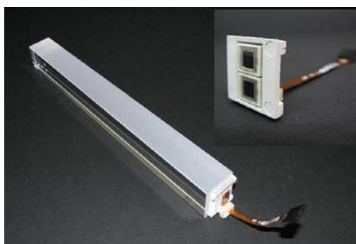
FIGURE 3.1: \text{PbWO}_4 crystal with APD photodetectors attached. The inset shows a capsule with two APDs. Figure from Ref. [11].
