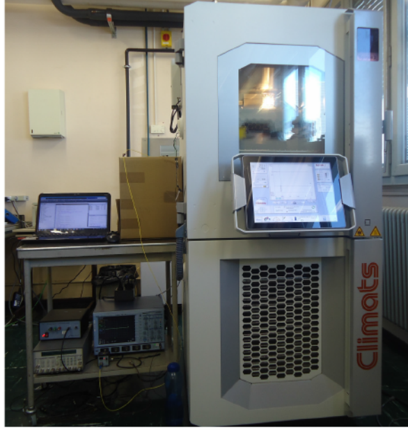
Figure 3: The chiller unit with the Oscilloscope, Function generator, Optical Box and Power supply.
