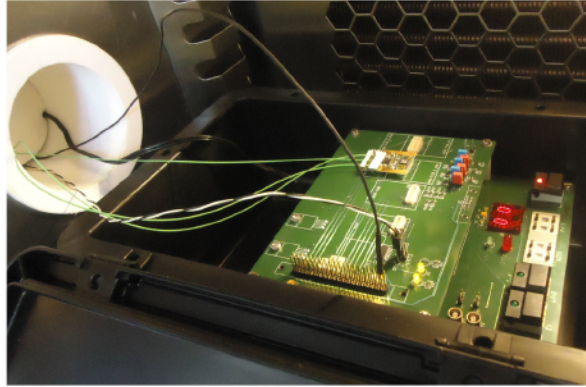
Figure 4: The test board with AOH board, optical lines and I2C lines.
