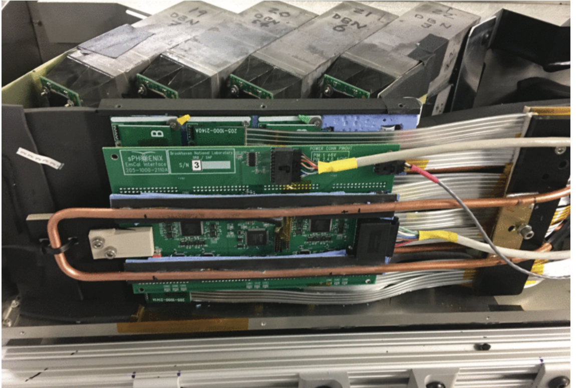
Figure 3.5: EMCal blocks (back), light guides, SiPMs, electronics (front), and part of the cooling system (copper pipe) as used for the beamtest. Taken from Ref. [53].
