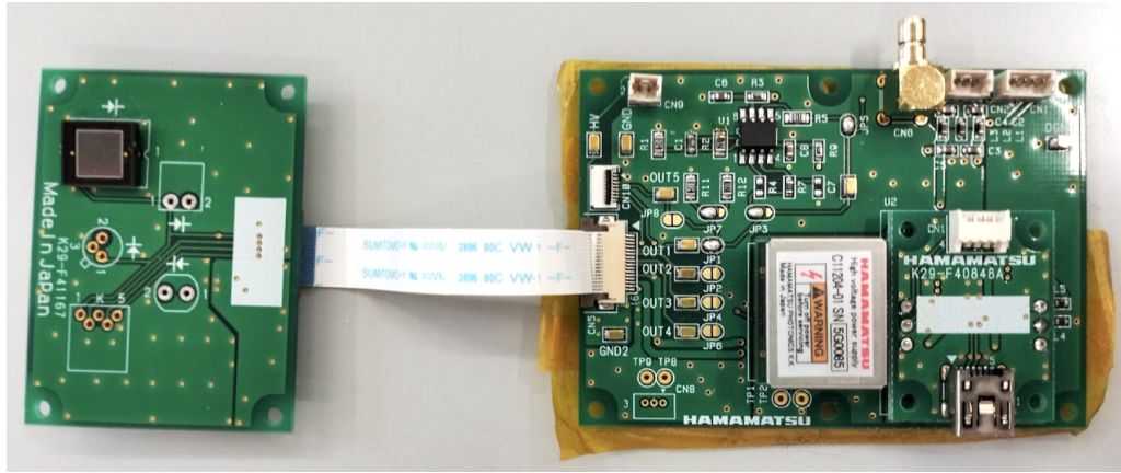
Figure 4.4: Photo of the Hamamatsu SiPM (left) connected to its powering board (right).
