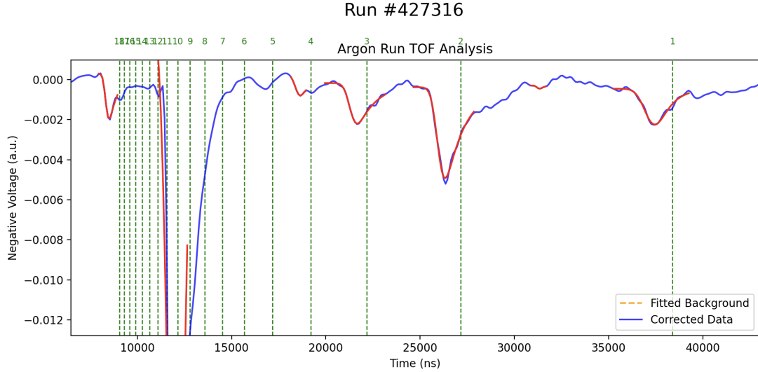
Figure 10: Run data with EMG (exponentially modified Gaussian) fitting
