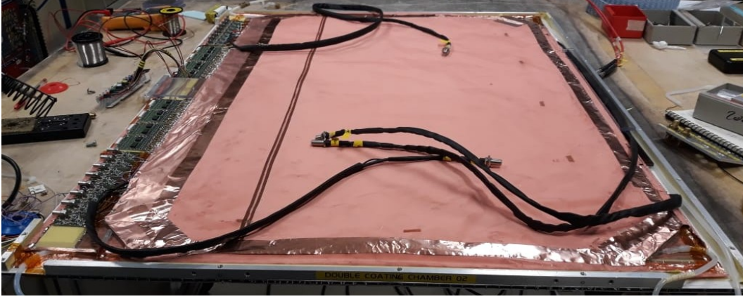
Figure 3.8. . Full assembled double coated graphite iRPC chamber at the B. 904 at CERN
