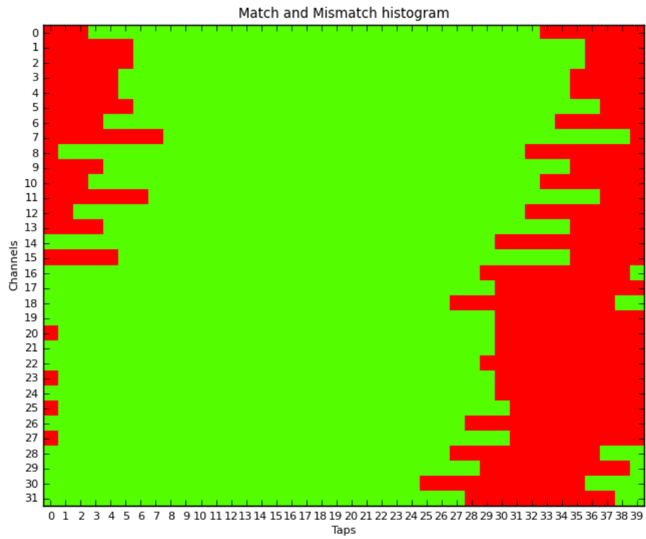
Figure 6.5: Phase scan of the received data from the MUCTPI installed in USA15
