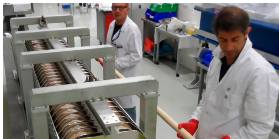
Experts of the TE-ABT group are working on the upgrade of the kicker magnets. In this picture, they have just removed the ceramic tube that contains the screen conductors from the magnet.
