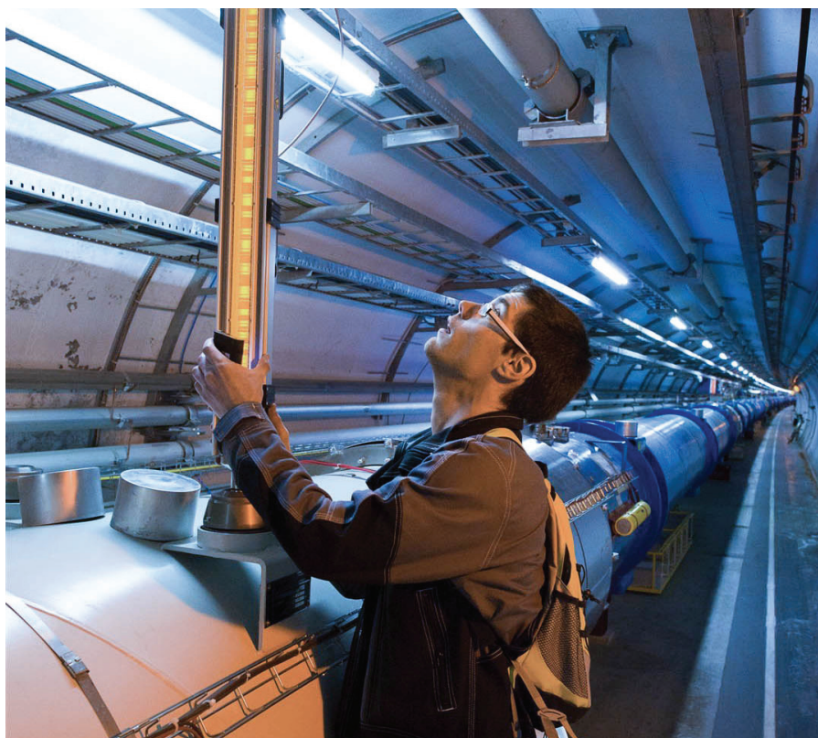
CERN surveyors take levelling measurements of the LHC magnets during LS1.
