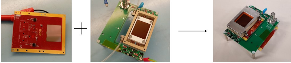
Figure 10: Images of the assembly of the triple-GEM on-top of the Timepix4 readout system. Timepix4v1 on the left, triple-GEM on the right, with the assembled detector as the result.
