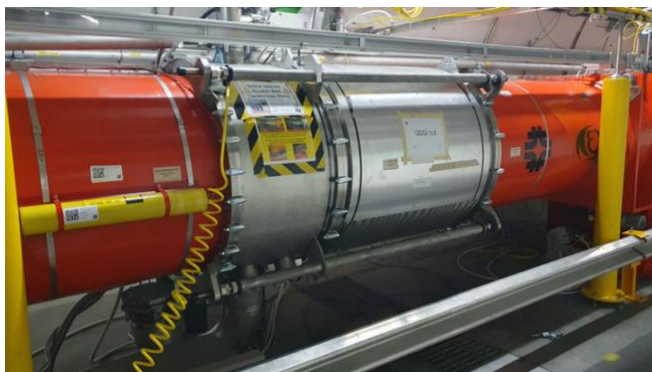
The interconnection between the Q1 (left) and Q2 (right) magnets when closed. (Image: CERN)
