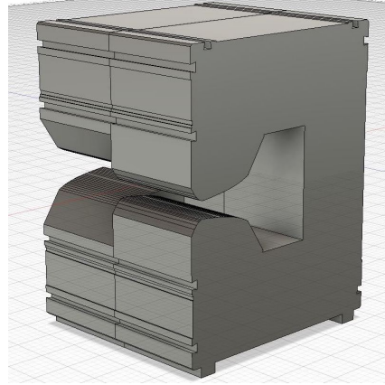
Fig. 1.1b The magnetic blocks (iron yokes) of the PS. This consists of a “closed” followed by an “open” combined function magnet. Taken from [13].
