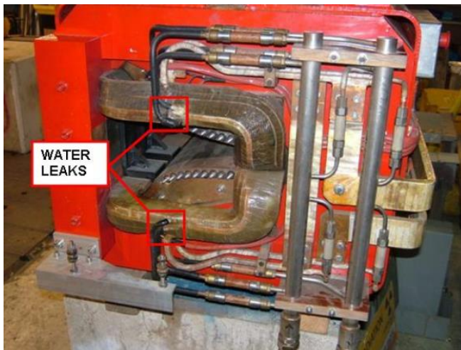
This picture shows the AD quadrupole where the water leak was situated. This is a half quadrupole that simultaneously generates a dipolar field to deviate the antiproton beam and a quadrupolar field to focus the antiprotons. (Image: CERN)
