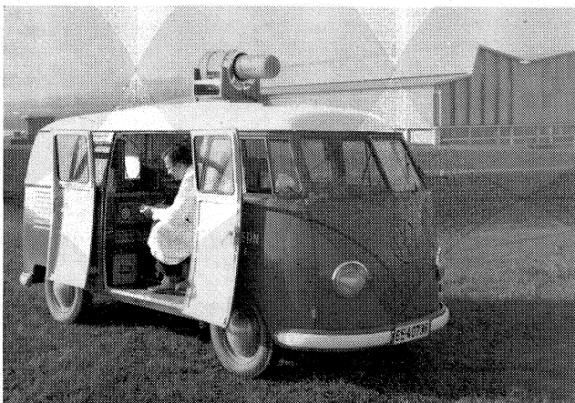
Sven Larson measuring the level of radio-activity on the mound covering the PS, by means of the apparatus installed in the mobile laboratory belonging to the "Health Physics" Group.
