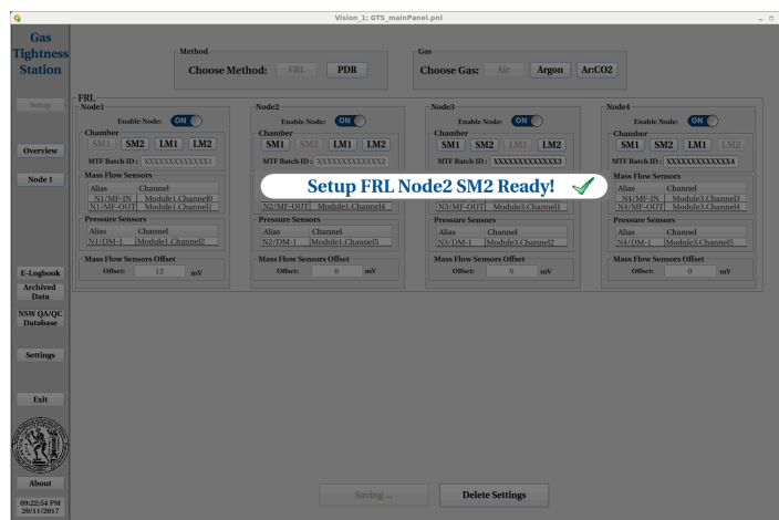
Figure 4.27: Automatically configure each node by pressing the Save Settings button and saving user-set settings.
