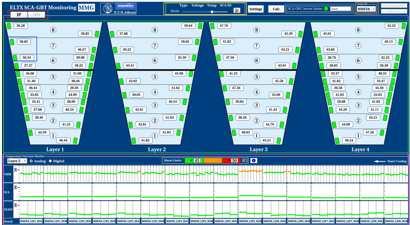
Figure 7.8: The main SCA DCS panel for Micromegas electronics monitoring.
