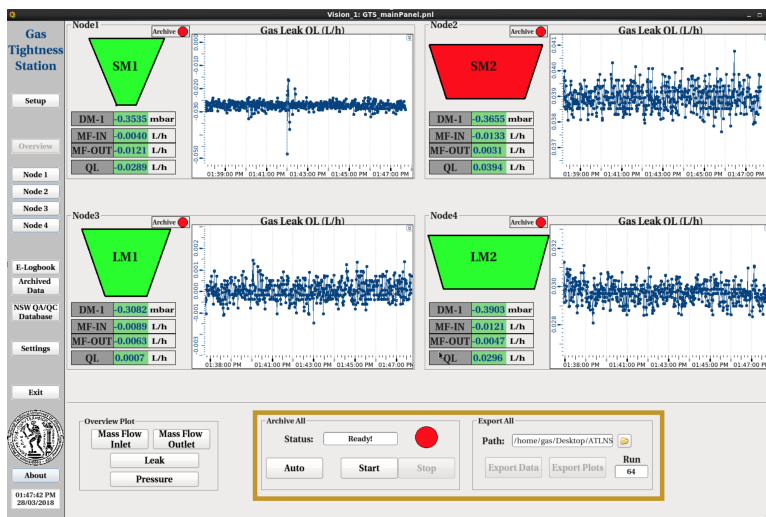
Figure 3.7: Archive/Export of all connected Nodes simultaneously
