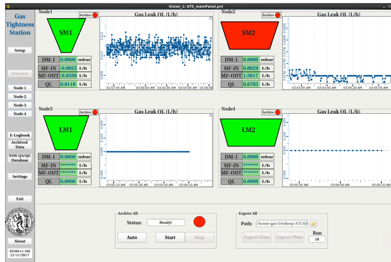
Figure 4.36: Check the sensors and MM QP of each node with 4-Node Mode in the FRL method.
