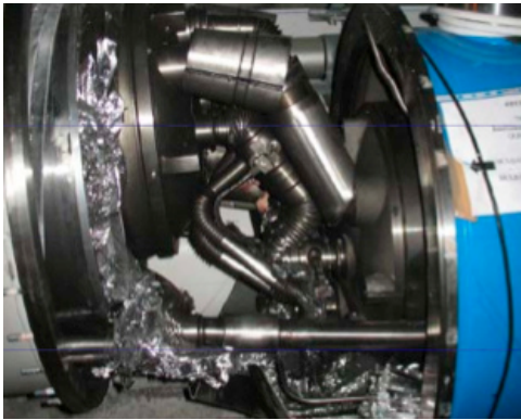
Figure 1: A severely damaged interconnect.
