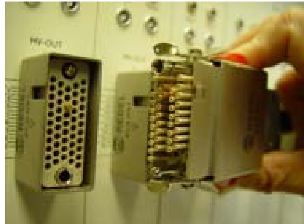
Figure 3.8: High-voltage cable connector and its counterpart on the HV power supply unit.
