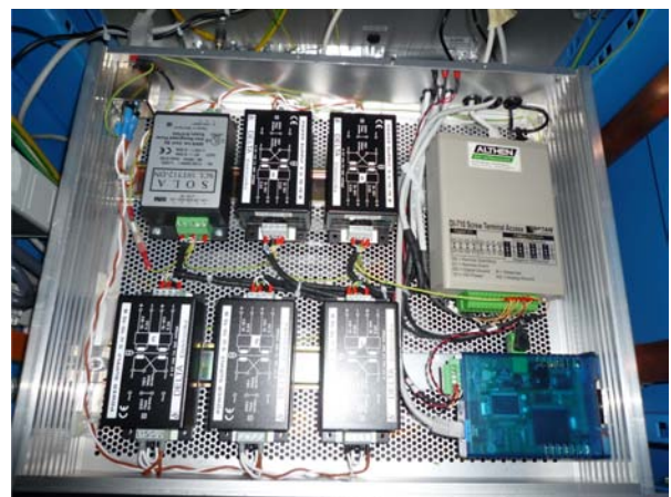
Figure 3.13: Return current data acquisition setup.
