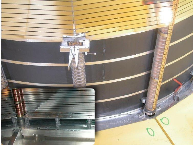
Figure 3.10: Picture of the inner field cage rods, field strips and inner containment vessel with guard rings. The inset shows field strips of the outer field cage and the skirts between the rods.
