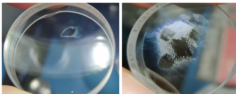
Figure 3.7: Deposits on mirrors with UV reflective coating caused by 200 ml of Styryl 8 (in ethanol and DMSO) and Rhodamine 101 (in ethanol) dye solutions in proximity to 50 mW of UV laser beam at 217 nm. After final assessment, it is clear that the deposits were caused by the DMSO in which the Styryl 8 had been dissolved.
