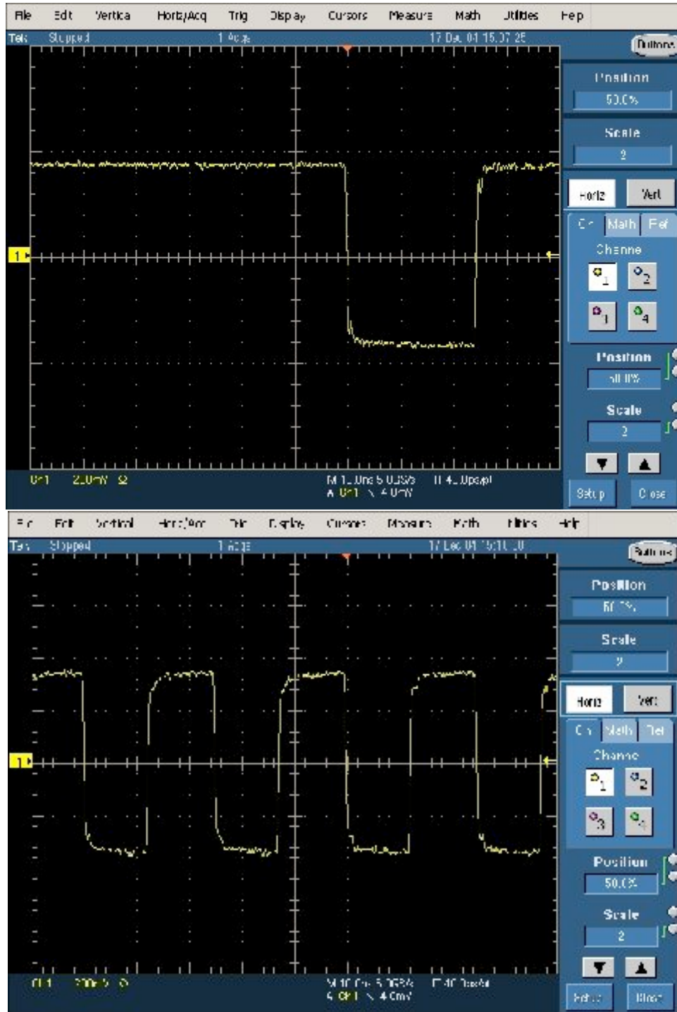
Figure 4.5: (a) This is part of a signal transmission to the CMM. The binary aspect of the signal can be seen as either being high or low. (b) The LHC clock signal. (Picture from N.Gee)
