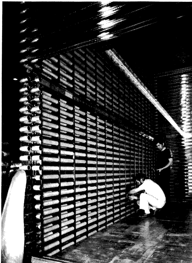
Inside the ISIS detector chamber during its assembly at CERN, showing the electrostatic structure and the horizontal plane of wires half-way up. (Photo 122.7.81)
