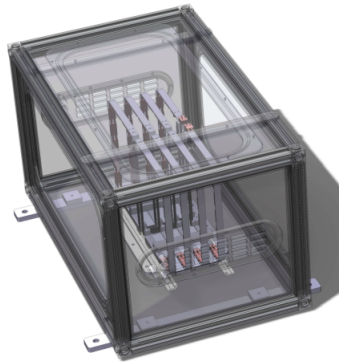
Figure 12.1: The computer model of Vertex Detector in NA61/SHINE. [25]
